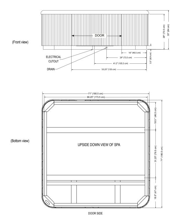
**NOTE:** Watkins Manufacturing Corporation recommends that the **SX** be installed on a minimum 10 cm thick reinforced concrete pad or structurally sound deck able to support the "dead weight" found in the spa specification chart.
