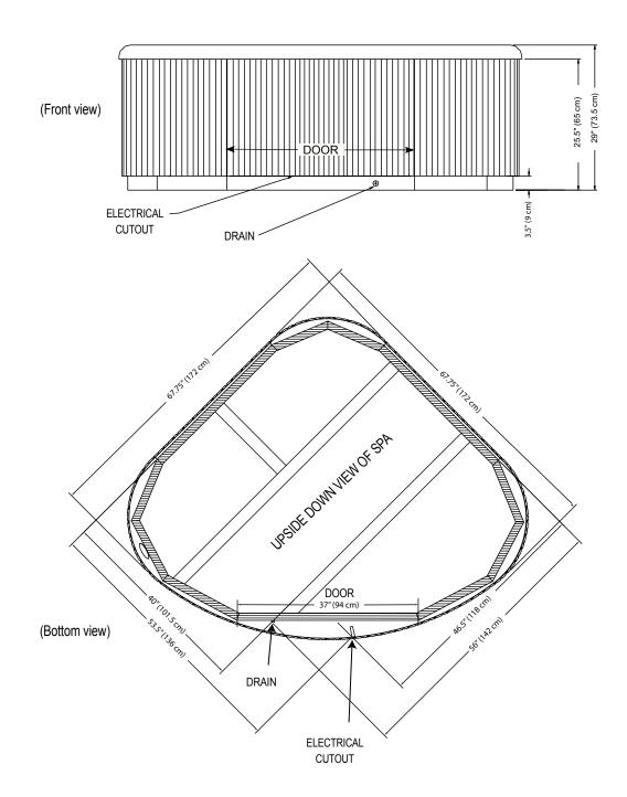
**NOTE:** Watkins Manufacturing Corporation recommends that the **TX** be installed on a minimum 10 cm thick reinforced concrete pad or structurally sound deck able to support the "dead weight" found in the spa specification chart.
