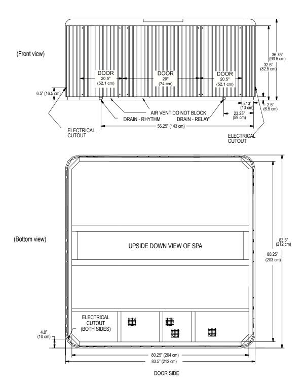
NOTE: Watkins Manufacturing Corporation recommends that the RELAY & RHYTHM be installed on a minimum 10 cm thick reinforced concrete pad or structurally sound deck able to support the "dead weight" found in the spa specification chart.
