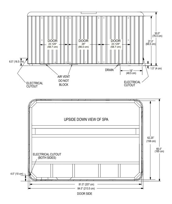
**NOTE:** Watkins Manufacturing Corporation recommends that the **STRIDE** be installed on a minimum 10 cm thick reinforced concrete pad or structurally sound deck able to support the "dead weight" found in the spa specification chart.
