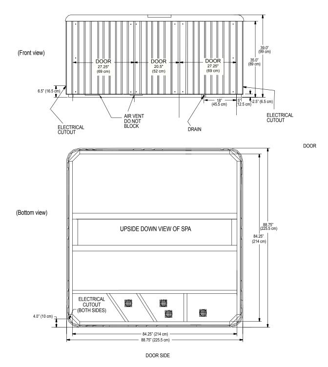
**NOTE:** Watkins Manufacturing Corporation recommends that the **TEMPO** be installed on a minimum 10 cm thick reinforced concrete pad or structurally sound deck able to support the "dead weight" found in the spa specification chart.
