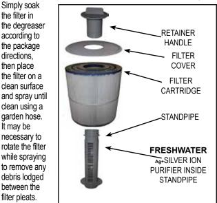
To reinstall the filter cartridge, reverse the order of steps in which it was removed. Do not overtighten.
